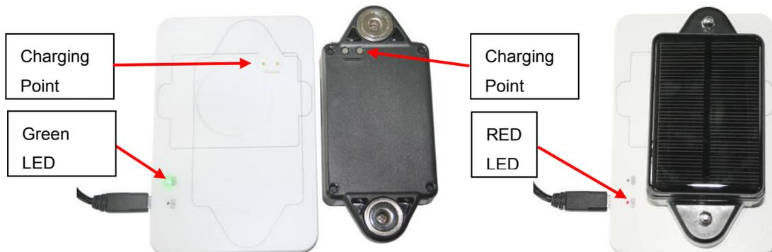
4.2 Use Solar Charging, Place the tracker in the sunlight, the solar battery will recharge the tracker automatically, in the long distance transport or longtime tracking please install the tracker in the place with sunlight, this can extend the battery working time, but it is impossible to finished fully charging only by solar power when working.
