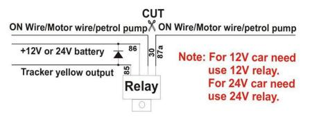
Attention: Turning off engine is very dangerous when car is driving, this will make the car difficult to control and maybe cause a accident, so we recommend make the relay cut the start motor wire, this will make you can not remote turn off car engine, but you can make the car engine can not be started
