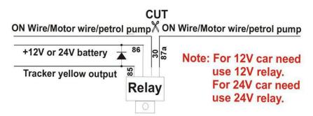
Attention: Turning off engine is very dangerous when car is driving, this will make the car difficult to control and maybe cause a accident, so we recommend make the relay cut the start motor wire, this will make you can not remote turn off car engine, but you can make the car engine can not be started
