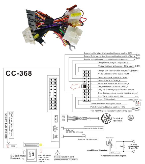
The immobilizer output can be used to control the car starting motor or oil pump motor line or ON line, etc. Please note a 30A relay need to connect to the immobilizer wire to control the engine off. The immobilizer output is an open-circuit negative output (load current 500mA), which can only drive the relay and cannot be directly connected to the circuit of the car. The relay is connected as shown below:
