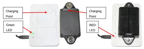
4.2 Use Solar Charging, Place the tracker in the sunlight, the solar battery will recharge the tracker automatically, in the long distance transport or longtime tracking please install the tracker in the place with sunlight, this can extend the battery working time, but it is impossible to finished fully charging only by solar power when working.
