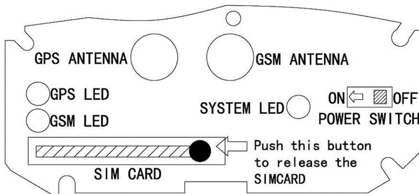
Map 1: Install the GSM SIM card, the GSM antenna and the GPS antenna
