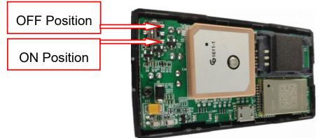
After power on the tracker will begin to work, the LED light will flash, first close the shell, put the tracker outside, after 5-10 minutes, see if the position of the tracker is updated, if the position has been updated, it means the tracker is normal.
