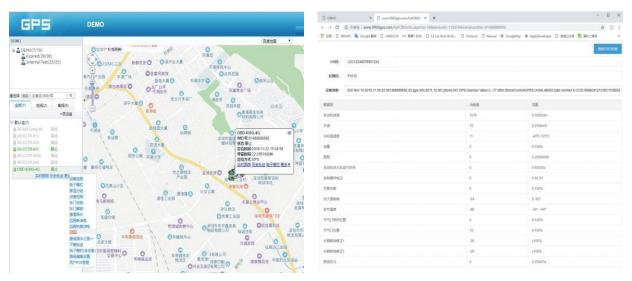
Note: OBD information query only supports web-side query, and does not support App query by now. Also due to different vehicle models, the read vehicle OBD information is also very different. Some models have only a few parameters can be queried, not all models cars can read.
